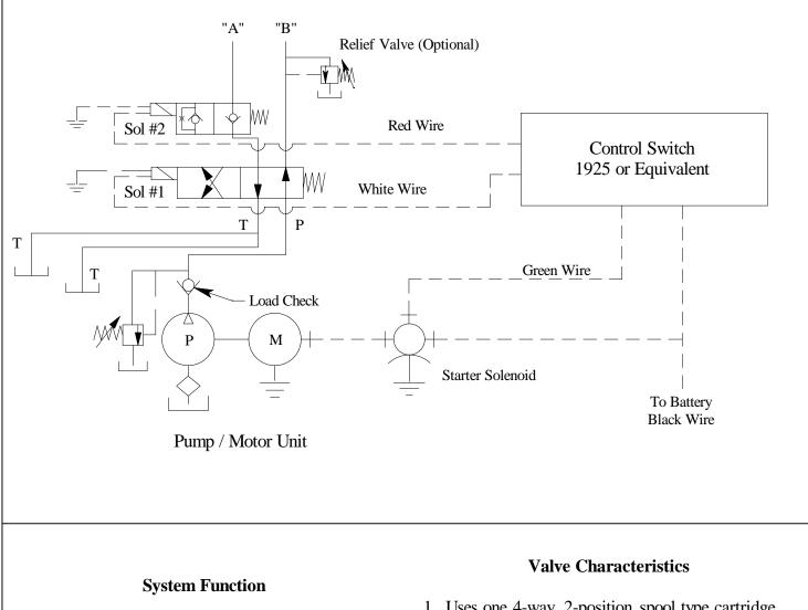
Energizing Power unit and Sol # 1, oil is directed to Port "A" and oil from Port "B" is directed back to tank ("T" Port).
