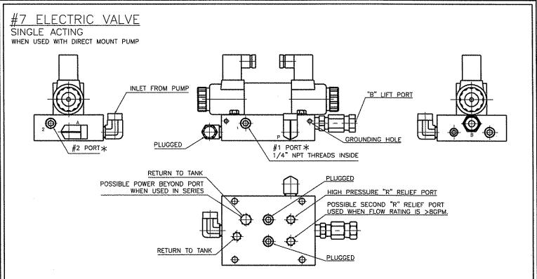
\* NOTE: AS WITH ALL WILLIAMS MACHINE AND TOOL VALVES, POWERING A SECONDARY VALVE IS POSSIBLE USING THE POWER BEYOND PORT ON THE BOTTOM OF THE VALVE. WITH THE ELECTRIC VALVES AN ALTERNATE POWER BEYOND PORT CAN BE ACCESSED ON THE SIDE OF THE SUB PLATE TO POWER ANY MISCELLANEOUS OPERTATION. REMOVING THE 3/8" NPT PLUG FROM THE #1 PORT AND INSERTING A 1/4" NPT PLUG AT THE BASE OF THE #1 PORT, ALLOWS THE #2 PORT TO BE USED AS A POWER BEYOND PORT AND THE #1 PORT TO BE USED AS A RETURN.
